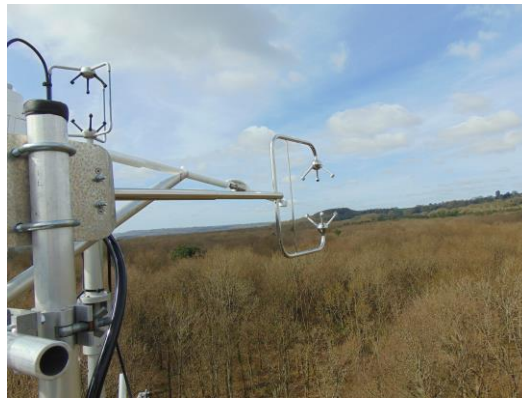
Eddy covariance instruments on the Alice Holt flux tower
